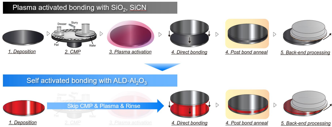
Figure 2. Self-activated bonding scheme omitting the pre-treatment steps (CMP/Plasma/Rinse)
